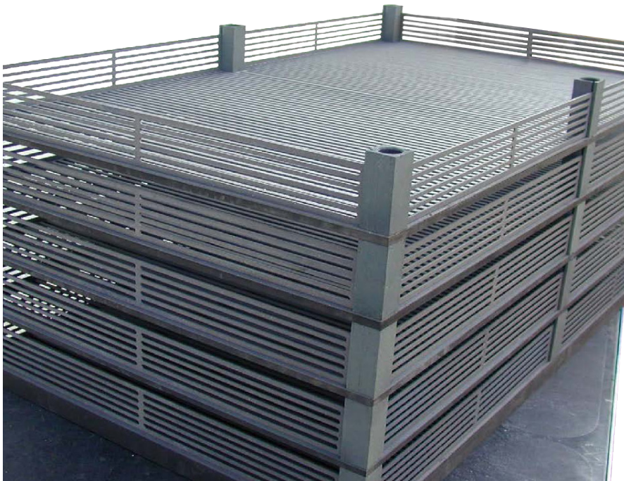
Assembly of Charging Boxes- CFC Performance
